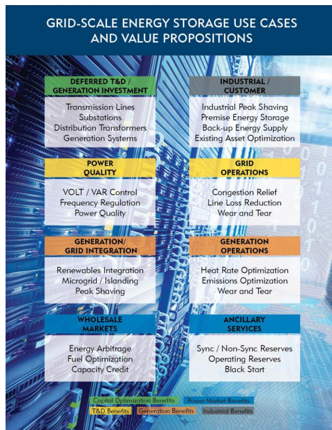
Figure 4-1: Potential Use Cases and Value Propositions of Grid-Scale Energy Storage
